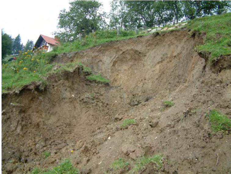
Fig. 3.2-3: Crater-like source area with the main scarp of a soil/debris flow, formed by excess pore water pressure (“soil explosion”). Photo source: GBA photo archives
