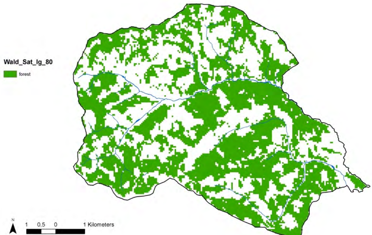
Fig. 5.3.1.3-9: Forest mask "Wald_Sat_Ig_80" based on the classification of satellite data after aggregation to 50 m with forest defined when at least 20 out of 25 pixels are classified as forest
