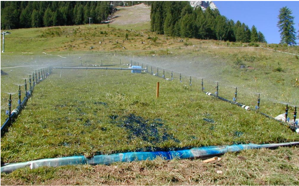
Fig. 4.3.4.1: Even on plots appearing quite homogenous to the human eye, surface flow concentrates within a short distance in deep lines. On sloped ground sheet flow changes to linear flow after a few meters.
